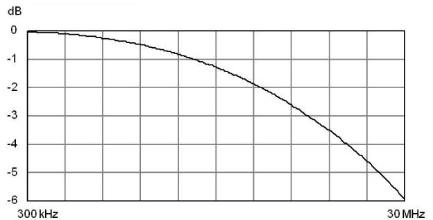
40-541-021 Insertion Loss Plot (typical worst case)
